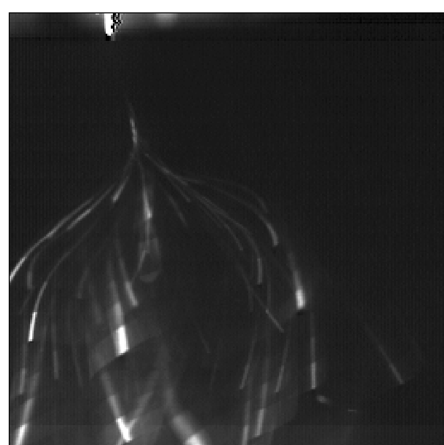
Electrospinning of PEO observed at 30 fps
