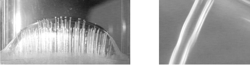
Figure 3: Freezing of water from the cooled bottom. Growing inclusions and close-up of their single structure.
