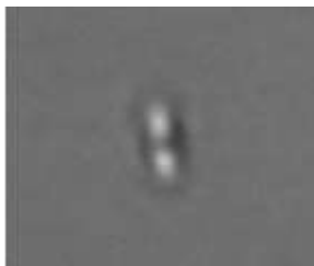
Figure 4.1. A short fiber trapped by the optical tweezers. The refractive index of the medium is 1.43, and the object index of refraction is 1.52.
