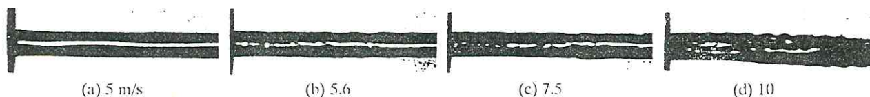
Fig. 2 - Ether jet, D = 100 \mu\text{m} , P_s = 58 \text{ kPa} , P_{\infty} = 100 \text{ kPa}
