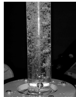
Fig. 2. Vibrational injection of gas into fluid
