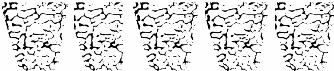
Fig.1. Graphically rebuilt micro-CT slices – an input for the adaptive mesh generator
