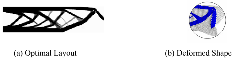
Fig. 1 An optimized result by a direct application of the element-density based topology optimization formulation for an end-compliance topology optimization considering geometrically nonlinear deformations.
