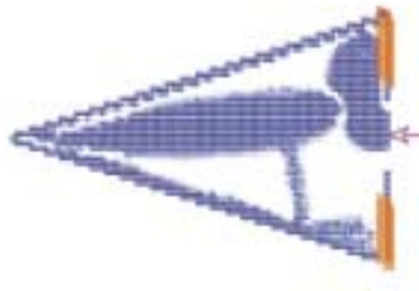
Figure 2. The optimized flap mechanism in undeformed configuration.
