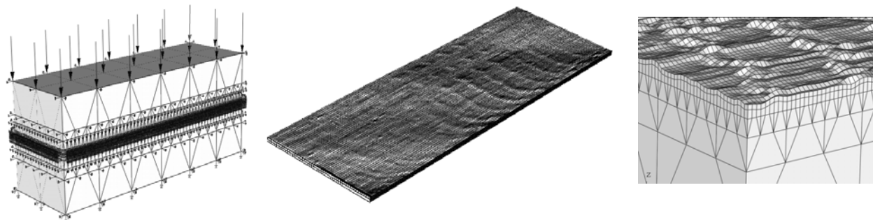
model with loads and constraints
