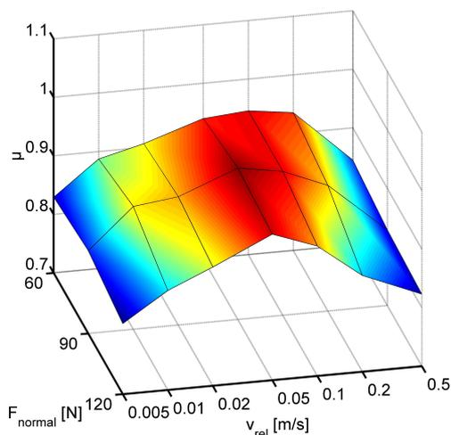
**Figure 2:** Friction coefficient field (wet road)
