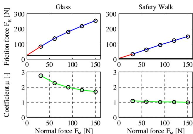
**Figure 3:** Friction force and friction coefficient versus normal force
