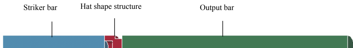
Fig.2 : Dynamic hat-shape structure test employing a direct Hopkinson pressure bar device
