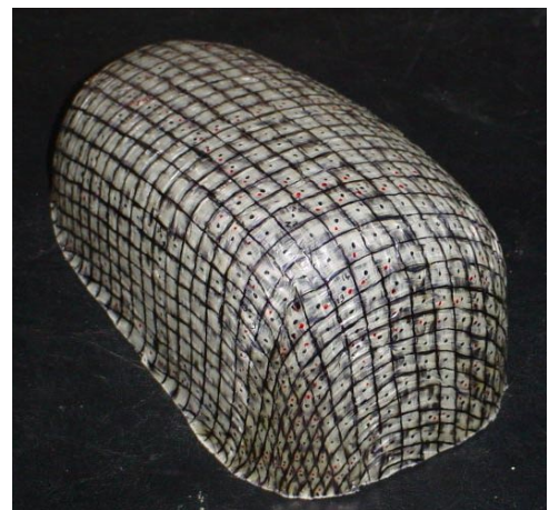
Figure 2: Car wing mirror holder formed from Twintex.
