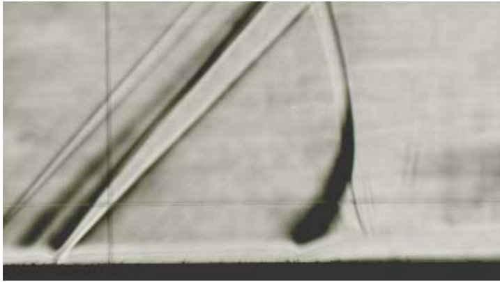
Fig.2. Shock wave and AJVG in operation, M=1.45
