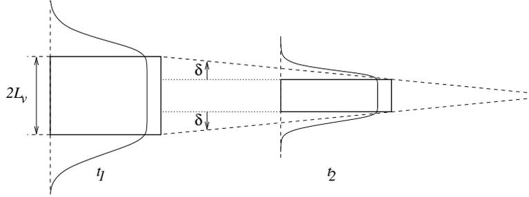
**Figure 3.** Schematic diagram of the two boundary layers during the slimdown regime.
