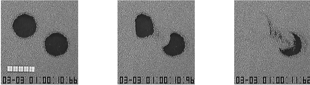
Fig.3. Collapse of two circular cavities. Initial radius R_0 = 18 mm, center-to-center distance l = 3R_0 , and angle of attack 30^\circ . Granular material is glass beads of a diameter 1mm.
