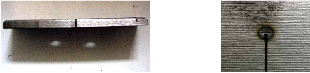
Fig2. The specimen and the state around crack tip after discharging
