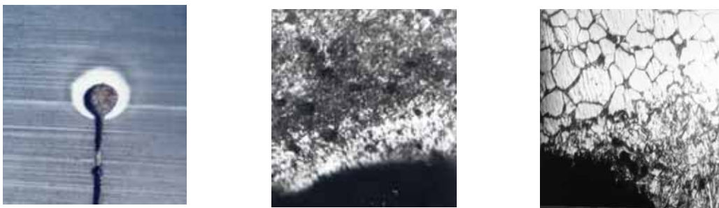
Fig1. White-bright layer macroscopical appearance and microstructure around crack tip
