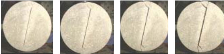
Fig.6 crack propagation trajectory of Brazilian disk specimens
