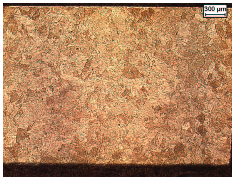
Figure 3. Austenitic grain of steel A after 10h at 1000°C ( \approx 100\text{--}150\ \mu\text{m} in diameter)
