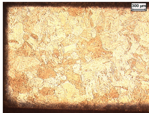
Figure 4. Austenitic grain of steel A after 10h at 1000°C ( \approx 200\text{--}300\ \mu\text{m} in diameter)
