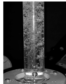
Fig. 2. Vibrational injection of gas into fluid
