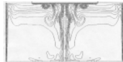
Fig.4. Instantaneous thermal's structure for buoyancy-driven convection, adiabatic melt surface, Pr = 6.5 , Gr = 4.5 \cdot 10^7 .
