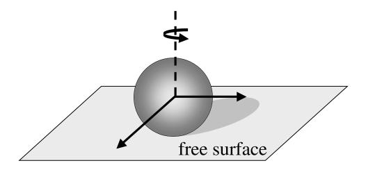
Three degrees of freedom of a sphere, which touches the planar free surface.
