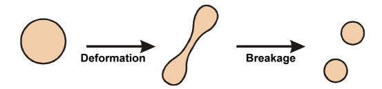
2. Necessary condition for drop breakage in inertial turbulent flow - the amplitude of the spatial fluctuations of the turbulent pressure is equal to the capillary pressure of the drops
