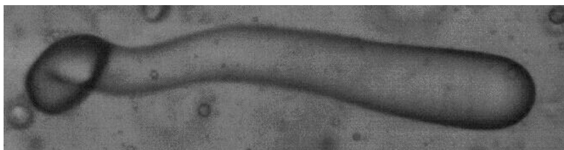
Different drop shapes observed in the space just after the processing element; (A) Bulgy type; (B) Lenticular type and (C) Cigar-type.
