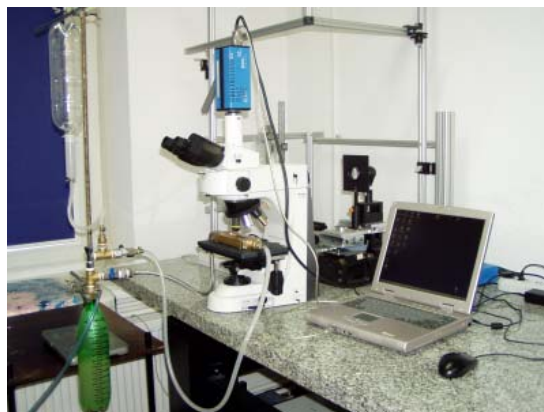
Figure 4. Photo of the experimental setup for micro PIV technique measurements and drops break-up process investigation, made up of Nikon Eclipse50i microscope, PCO1200hs high speed camera (for drops observation; for PIV measurements was used other camera: PCO Sensicam), pressure system for flow acceleration and PC computer for data acquisition.
