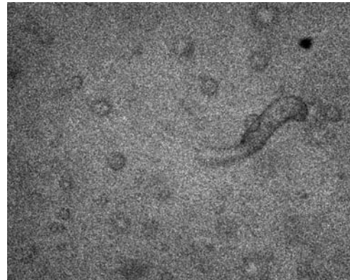
Figure 2.11. Result for S50 oil – emulsion with 1%wt SDS surfactant; oil drops 2mm behind processing element and 0.4mm below glass wall ( x = 2 , y = -0.4 ); velocity of the droplet v_d = 4.7m/s ; figure width corresponds to 432\mu m .
