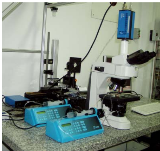
Figure 5. Photo of the experimental setup for investigation of jet break-up process; pressure system replaced with two precision syringe pumps
