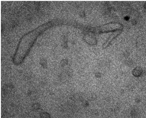
Figure 2.11. Result for S50 oil – emulsion with 1%wt SDS surfactant; oil drops 2mm behind processing element and 0.4mm below glass wall ( x = 2 , y = -0.4 ); velocity of the droplet v_d = 4.7m/s ; figure width corresponds to 432\mu m .
