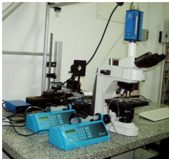
Figure 5. Experimental set-up for investigation of jet break-up process; pressure system is replaced with two precision syringe pumps.
