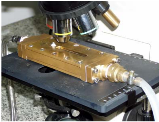
Figure 6. Emulsifier model installed under microscope.
