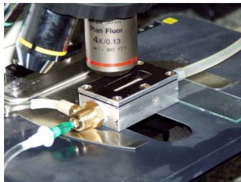
Figure 9. Experimental chamber for investigation of break-up process of liquid jet in co-flow installed under microscope.
