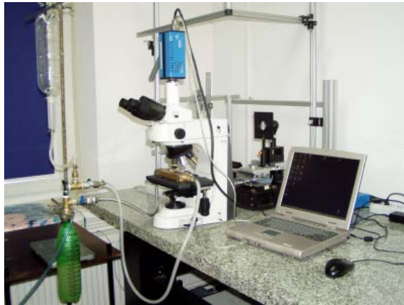
Figure 4. Experimental set-up for micro PIV technique measurements and drops break-up process investigation: Nikon Eclipse50i microscope, PCO1200hs high-speed camera (for drops observation; for PIV measurements are used other camera: PCO SensiCam), pressure system for flow acceleration and PC computer for data acquisition.
